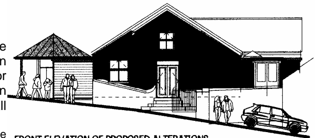
FRONT ELEVATION OF PROPOSED ALTERATIONS NEW ENTRANCE CANOPY ON LEFT NEW LINK BLOCK ON RIGHT
